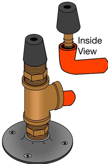
3. Thread the brass nipples (part # 8) into each end of the tee. The hose will extend through the top nipple.
