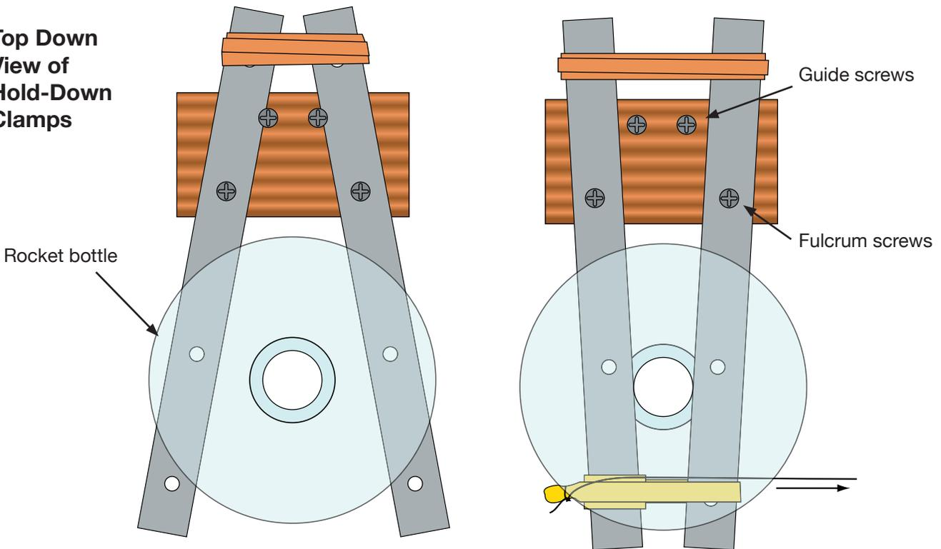
**Placing the hold-down clamps (8" mending plates)**
